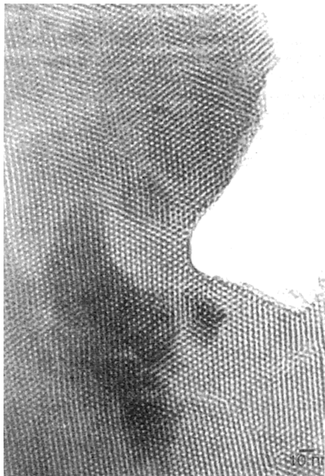
Figure 2. TEM of a calcined hexagonally ordered zirconium oxophosphate. Reprinted with permission from ref 3. Copyright 1999 Elsevier.
